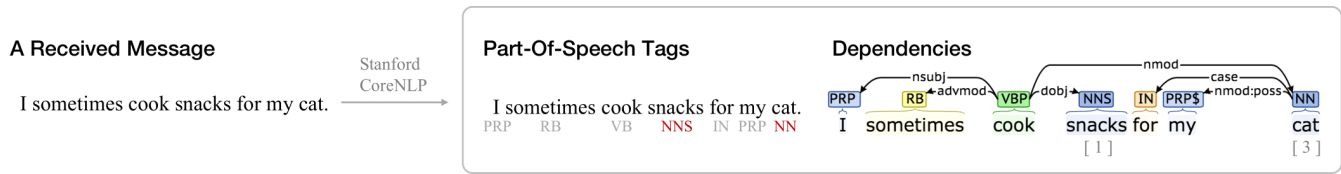
Figure 2: Our computational pipeline combines Part-of-Speech tagging and dependencies to select a noun by assigning weighted probabilities based on the degree ( i.e. , the number of edges) of each noun.
